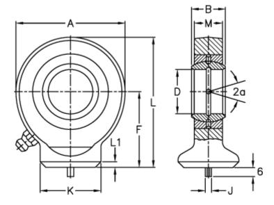
$\begin{array}{lll} A & = 180 \\ a \ (degrees) & = 6 \\ B & = 55 \\ D & = 80 \\ Dynamic load C \ (kN) = 400 \\ F & = 141 \\ J & = 6 \\ K & = 95 \\ \end{array}$
